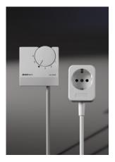
Plug thermostat: The plug thermostat is simply installed between heating and socket and is particularly suitable for mobile heaters. Its integrated sensor measures the room temperature and accordingly regulates the heat output. Like all our thermostats, the plug thermostat is provided with frost protection that is activated when the temperature reaches 5 °C.
